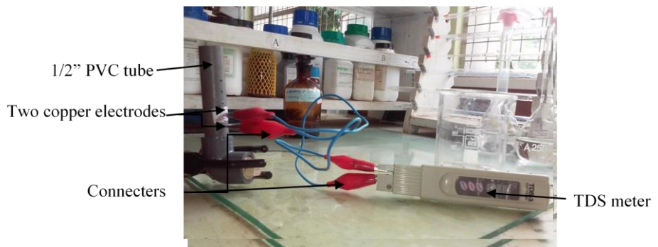
Figure 4. Calibration of online TDS monitor
